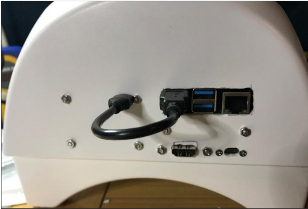
Figure 5: Peripheral interface for the dispenser.
